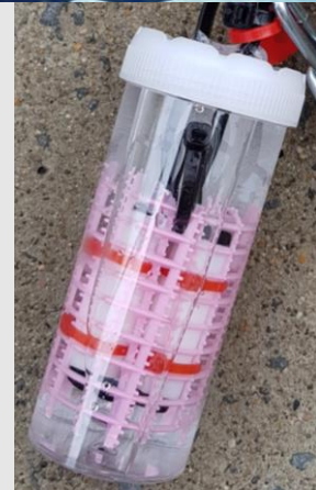
Passive sampler tubes in deployment mesh
